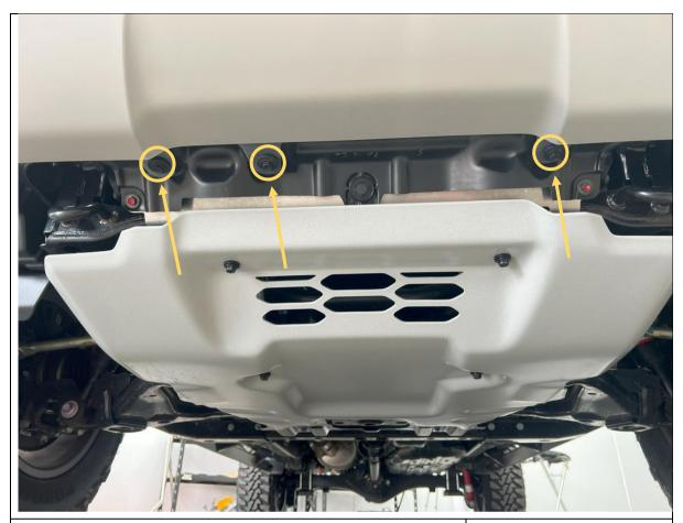
15. Remove the 3x Factory Screws securing bottom center section of bumper to inner wheel arch liner. Use 10mm socket / spanner.
