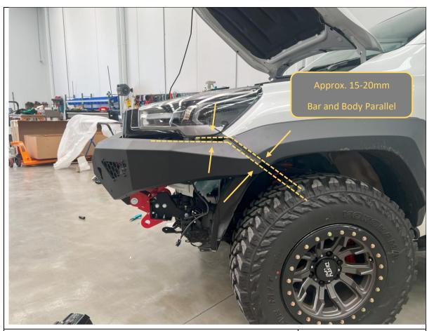
95. Align the bar with the body. Aim for 15-20mm clearance between the wing and body.
