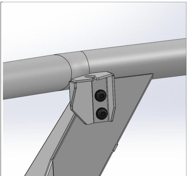
127. **Toro only.** Fit antenna brackets to Toro uprights using M8x20 black button head bolts and black washers.
