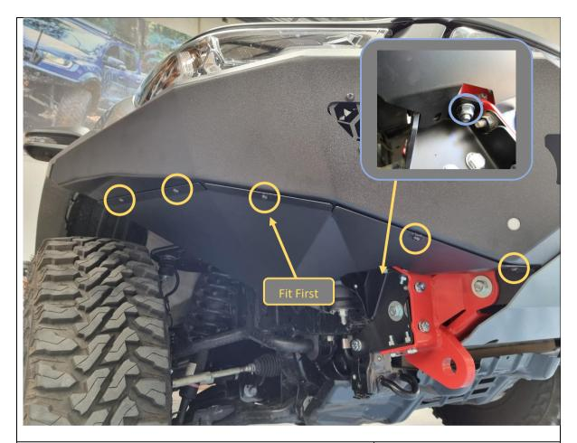
120. Fit side under panels to bar and secure with 5x M6x16 Button head bolts and M6 Flat washers, into M6 cage nuts fitted earlier.
