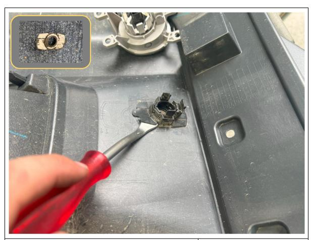
58. Carefully pry the sensor housings away from the back of the bumper, using a trim tool or similar.
