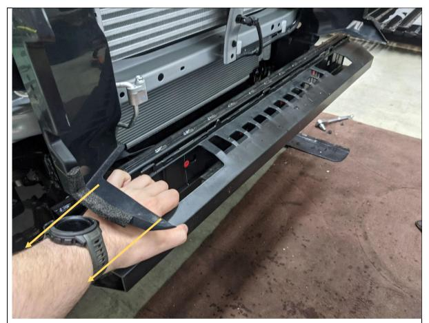
31. Remove the plastic cover from the impact beam by strongly pulling in the direction shown to release it from the clips
