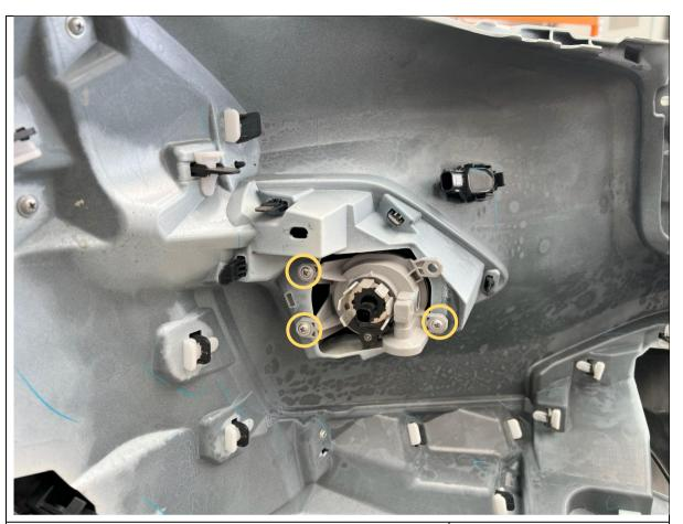
56. Remove the 3x Screws securing the fog lights to the bumper, then remove the fog light from the bumper.
