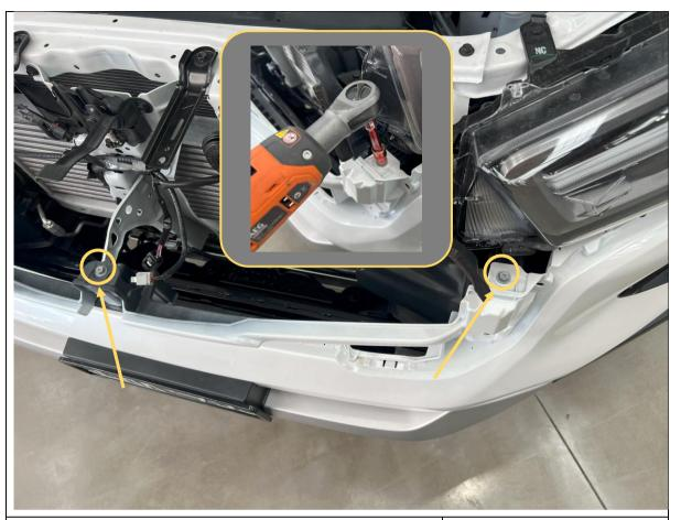
19. Remove the 3x 10mm Head/Phillips screws securing the bumper to crossmember.
