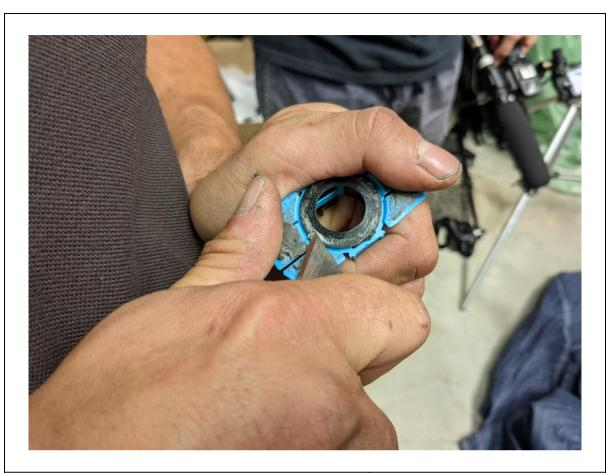
59. Remove remnant adhesive from the face of the sensor housing, using a utility knife and / or solvents.
