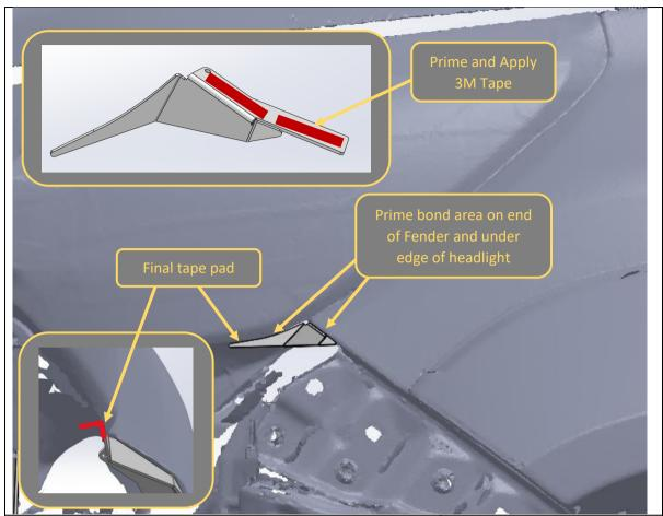
82. Using 3M primer stick from parking sensors, apply primer to end of fender panel and small headlight infill in the bonding area as shown.
