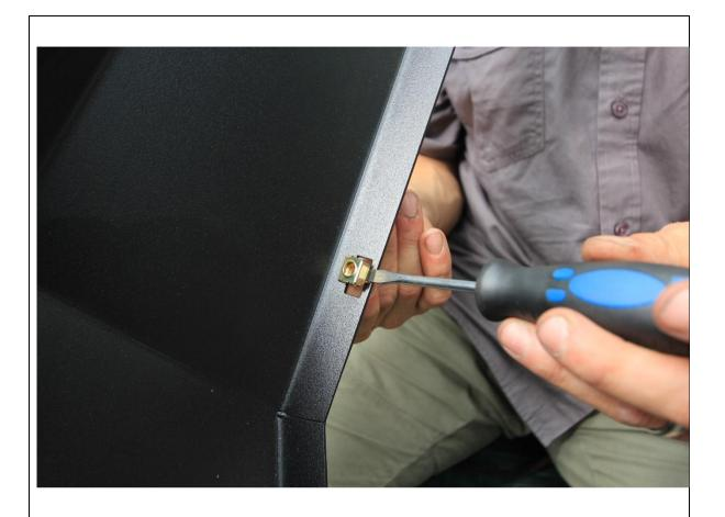
91. Insert cage nuts to square slots in bottom of wings. Seat cage nut against one edge of slot then push other edge in with flat bladed screwdriver.
