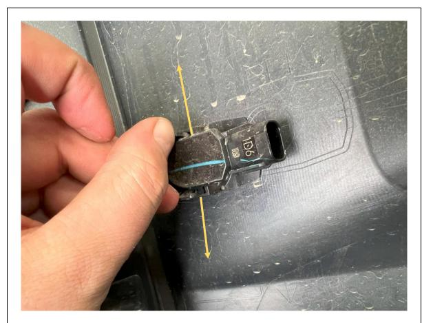
57. Remove parking sensors from housings, by prying apart the locking tabs, whilst pushing sensor from front side of bumper.
